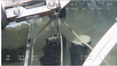
Figure 4. Casting of specimens for strength tests
