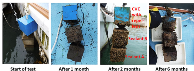
Figure 13. Specimens for marine biofouling
