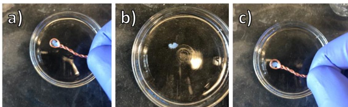
Figure 2–31. Optical images of SAMM multilayer film: (a) as synthesized, b) soaking in \text{H}_2\text{O} and (c) after exposure to \text{H}_2\text{O} for 2 h.
