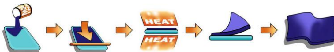
Figure 1–16. Process for formation of MMM. 52 A MOF-based ink is applied to a BYTAC substrate (Teflon resin surface protectors, purchased from Saint Gobain Performance Plastics) on a glass plate by bar coating to create a uniform film. The applied MOF-based ink is heated to cure the RTV615 A/B and remove solvent, producing the MMM on the substrate. MMM film is delaminated from substrate giving a freestanding MMM.
