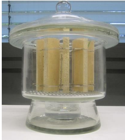
Figure 3-1. Photographs of the experimental setup for formaldehyde emission rates
