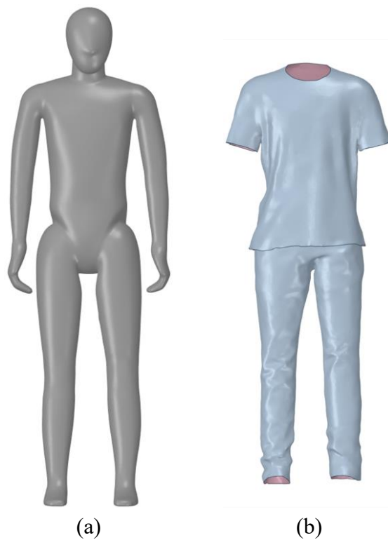
Figure 4-1. Three-dimensional (3D) digital model of thermal manikin and clothes: (a) Manikin and (b) T-shirt and Pants
