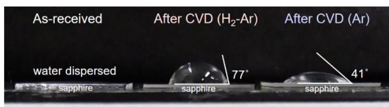
Figure 3.12. Water contact angle measurements for the pristine sapphire and the sapphire after the CVD with H 2 -Ar and pure Ar flows.
