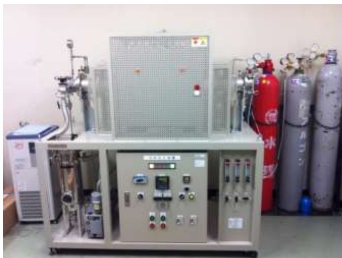
Figure 3.3. High temperature vacuum furnace for \text{H}_2 treatment.
