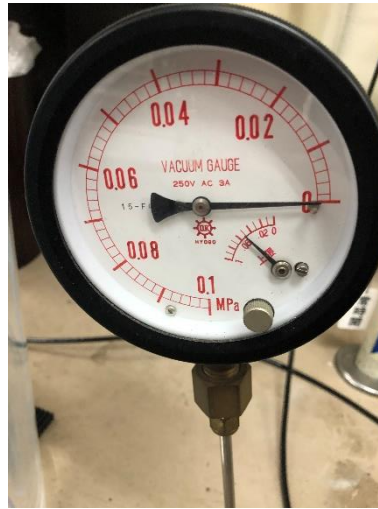
Fig. 4.9 The output view of the pressure meter. The meter dial accuracy was 0.002 Mpa. By using this pressure meter, the 3% CO 2 that injected into the gas chamber has an error of \pm 2\% .
