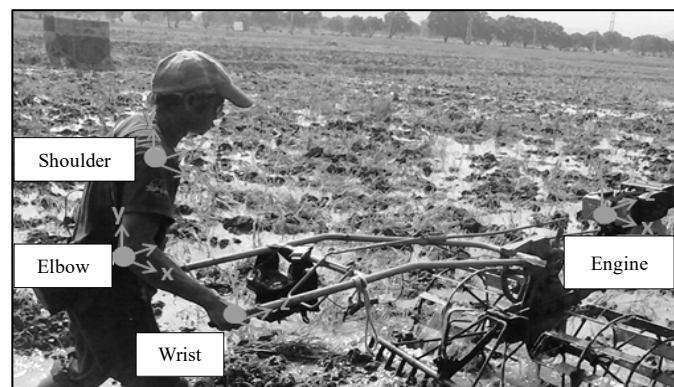
Figure 1.1. Measurement of vibration acceleration on the engine, wrist, elbow, and shoulder during actual hand tractor operation.
