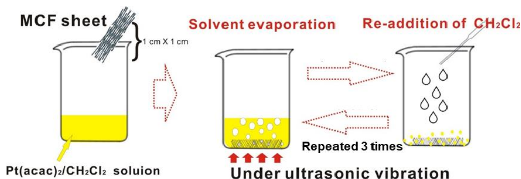
Fig. 2.8 A schematic diagram of the Pt deposition process on MCF sheet.
