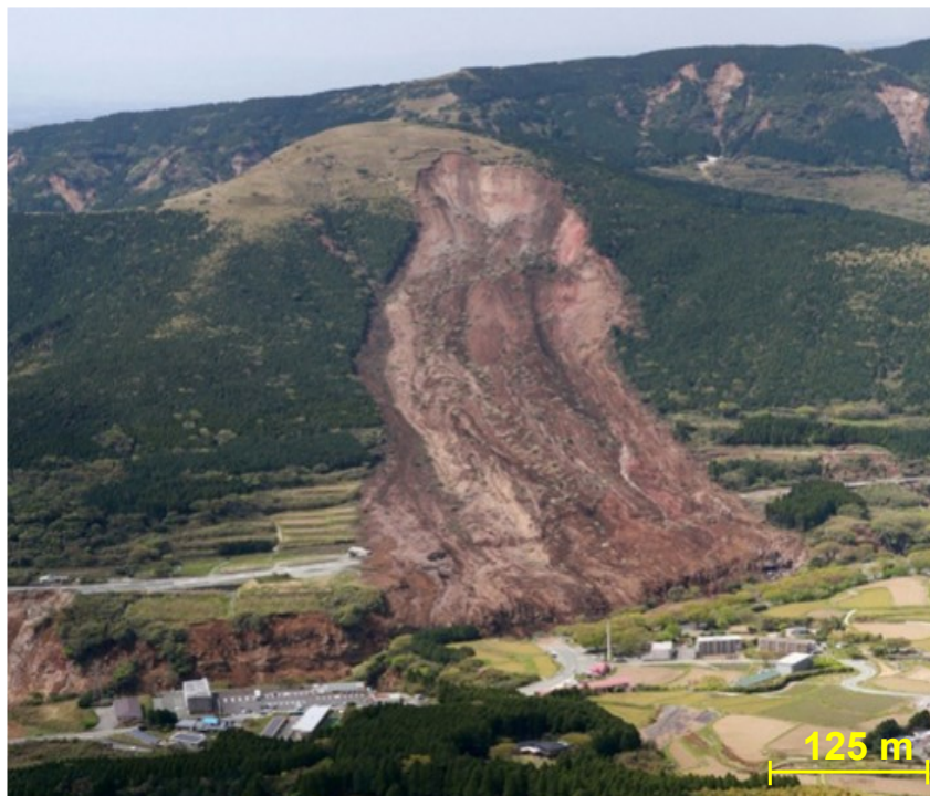
Fig. 1.2 Slope failure after Kumamoto earthquake April 2016, Japan ( https://mainichi.jp/ )
