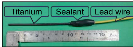
Figure 5.1 Schematic of embeddable titanium wire sensor (TWS)
