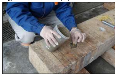
(c) Anode backfill material casting
