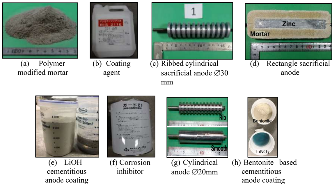
Figure 4.21 Material for repair process
