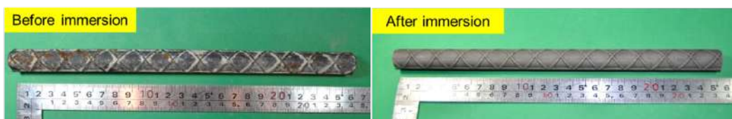
Figure 3.35 A 20-year-old deteriorated steel bar used in this study
