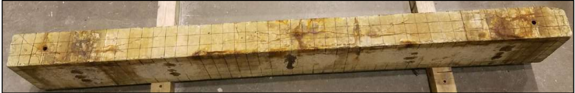
Figure 4.10 Appearance and cracking pattern of RC-3
