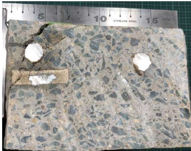
Figure 3.54 Cross-sectional area of the specimen with 10 \text{ kg/m}^3 of chloride content
