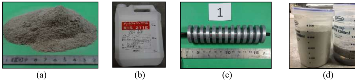
Figure 5.19 Materials for repair: (a) polymer modified mortar, (b) coating agent, (c) cylindrical ribbed sacrificial zinc anode and (d) Cementitious anode coating material mixed with LiOH
