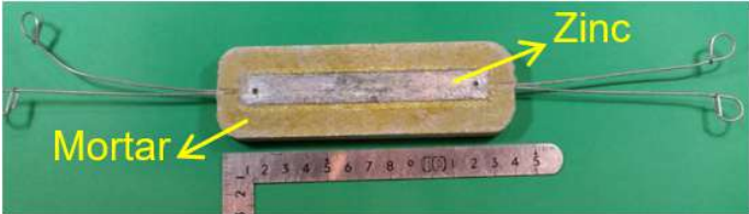
Figure 3.22 Sacrificial anode installed on the rebar (Rafdinal, 2016; Rafdinal et al., 2016)
