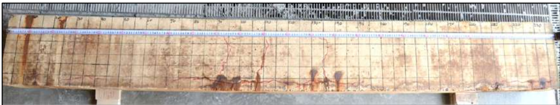
Figure 4.8 Appearance and cracking pattern of RC-1
