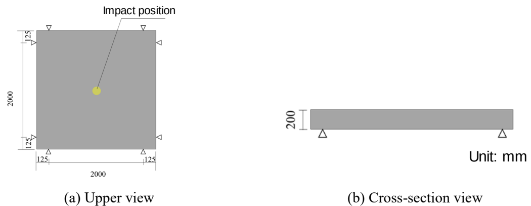
Fig 6.1 Size of the concrete model
