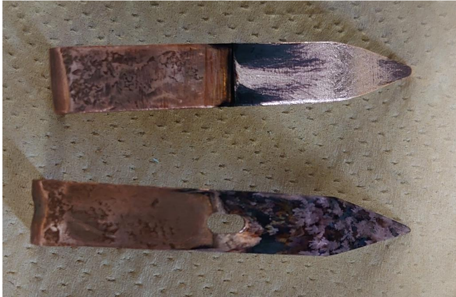
Figure 3.10. Anode (upper) and cathode (lower) appearance with contamination of carbon after experiment of normal shape solid propellant
