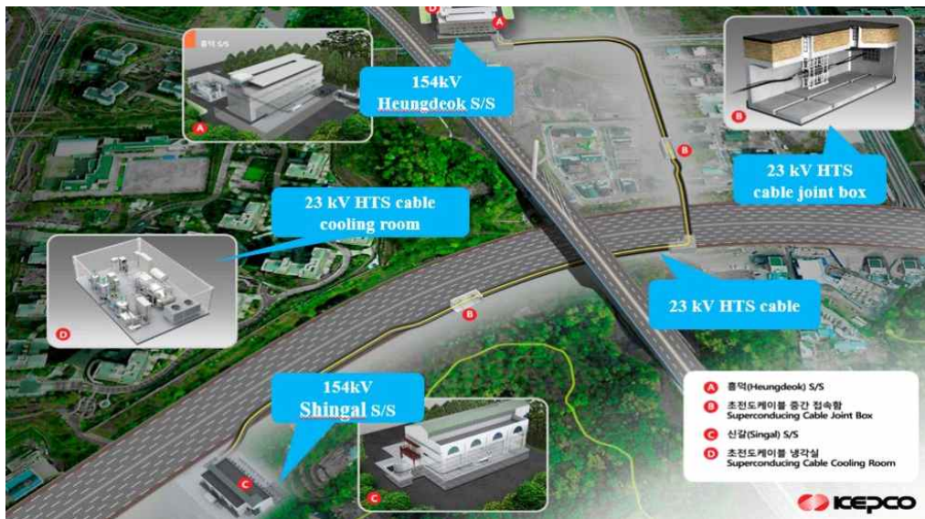
Fig. 1.10 A 23 kV HTS cable system configuration of the Shingal Project in South Korea
