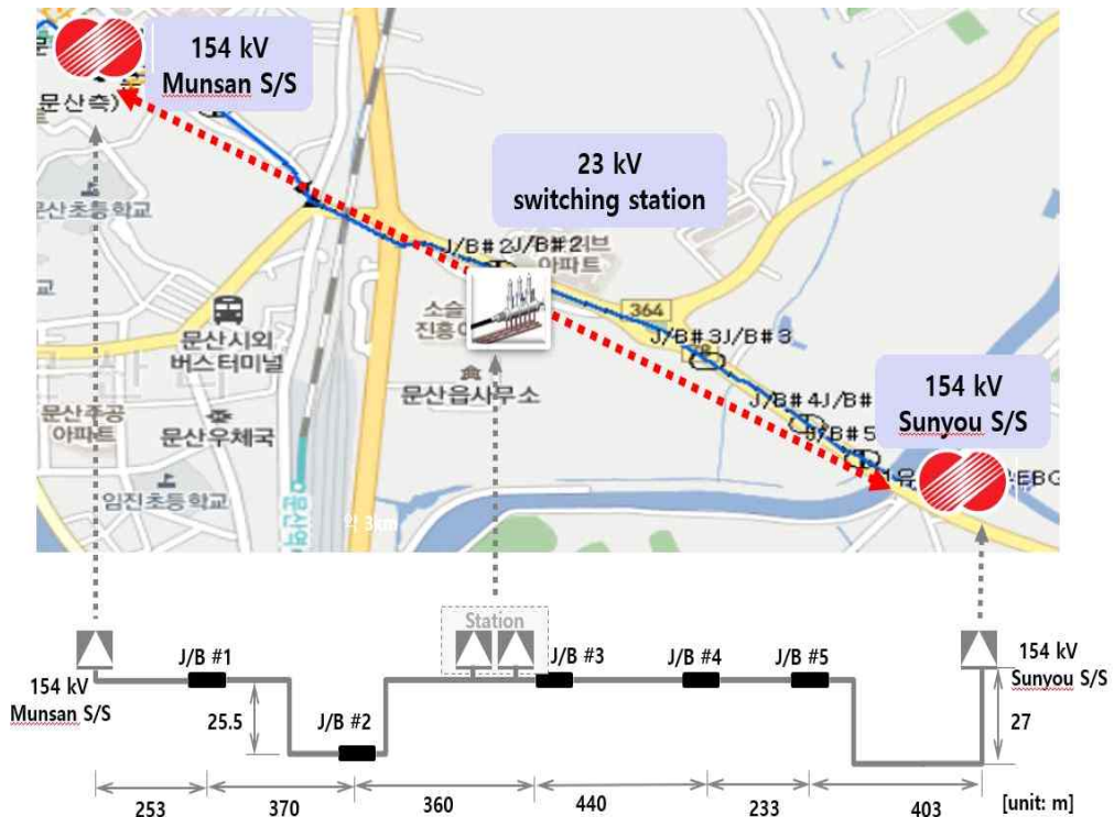
Fig. 5.2 The demonstration project of a 23 kV 60 MVA HTS power platform between KEPCO's 154 kV Munsan and Sunyou substations
