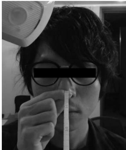
Figure 3.1. Procedure of Experiment 1 and Experiment 2. Measurements of viewing distances and angles, as obtained from the tip of the participant's nose to the middle of the three near-infra-red lights of the eye tracker used in Experiment 1, or to the midpoint in between the two near-infra-red lights of the eye tracker used in Experiment 2.
