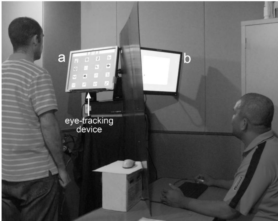
Figure 6.2. Impression of the experiment set-up of Experiment 6. a. The participant was standing in front of the monitor which showed the experiment interface. b. The experimenter controlled the order of password format, grid, and password length for the participant using another monitor.
