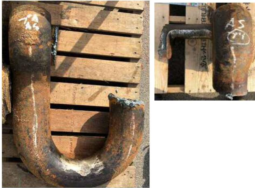
(b) Seafloor side mooring chain.
