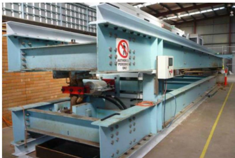
Fig. 1.6 Full scale wear rig as seen from test specimen end conducted by Jayasinghe 3) .
