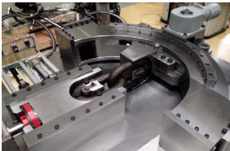
Fig. 1.5 Overview of mooring chain wear test setup conducted by Gotoh et al. 22) .
