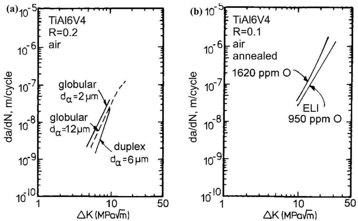
Figure. 1.24. Fatigue crack propagation rate in Ti-6Al-4V. (a) Effect of grain size in equiaxed and duplex microstructures [137], (b) Effect of oxygen in annealed condition [138].
