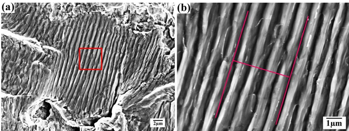
Figure 4.7. Fracture surface at 298 K,  $\Delta K = 26.5 \text{ MPam}^{1/2}$ , and  $R=0.1$ , (a). Striations at low magnification, (b) Spacing between striations that equals to  $da/dN$ .
