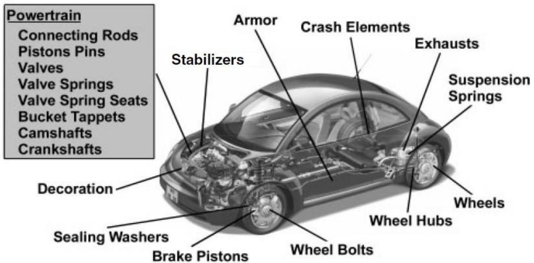
Figure 1.2. The possible applications of titanium for vehicles [34].
