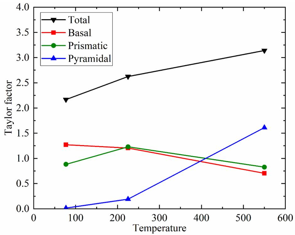
Figure 3.7. Temperature dependence of Taylor factor in each slip system.
