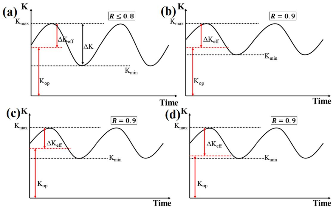
Figure. 4.10. The schematic of the change in  $\Delta K_{\text{eff}}$  and  $K_{\text{op}}$  levels at lower and higher  $R$  ratios.
