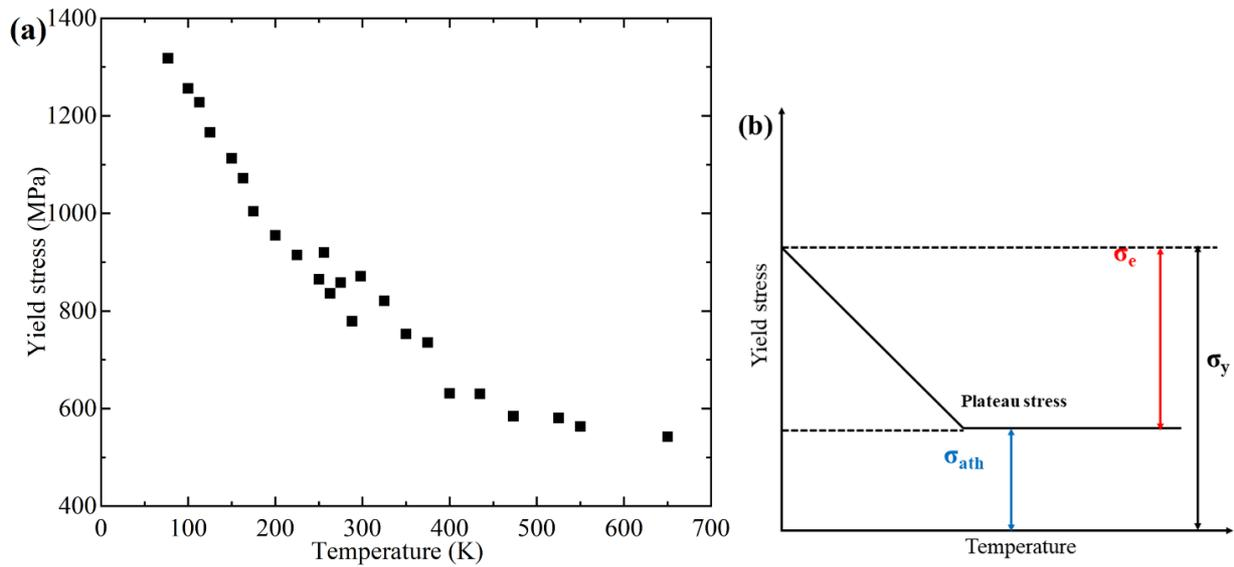
Figure 2.6 (a) Temperature dependence of yield stress obtained in this study. (b) Schematic drawing of the temperature dependence of yield stress.
