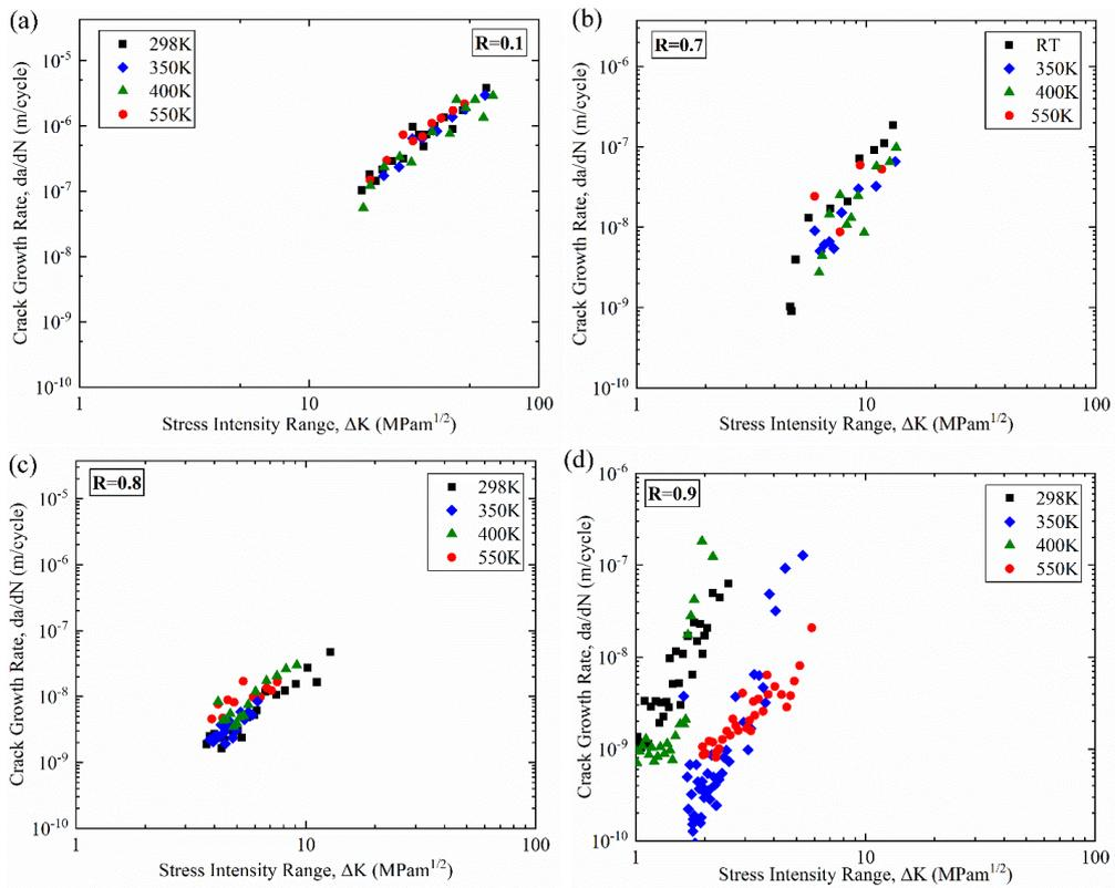
Figure 4.5. Fatigue crack growth rates of bimodal Ti-6Al-4V at various temperatures with different stress ratios. (a) R=0.1, (b) R=0.7, (c) R=0.8, and (d) R=0.9
