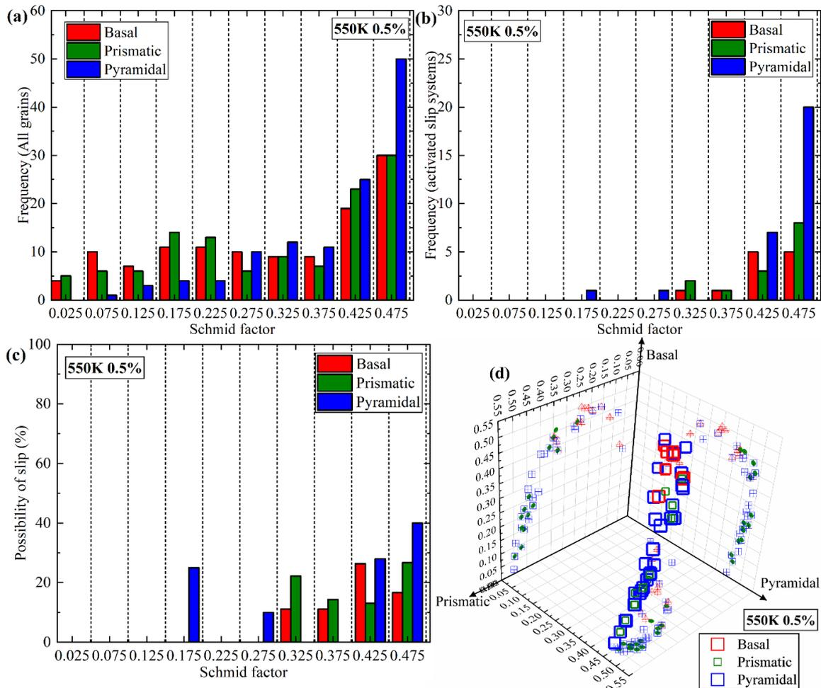
Figure 3.6. Consolidated histograms of Schmid factor for three slip systems at 550 K with the strain of 0.05. (a) for all grains, (b) for activated slip systems in deformed grains, (c) possibility of the slip activation, (d) Schmid factor distribution of activated slip systems in 3D. The projected symbols are different from those in Figs. 4 and 5 for the visibility in case of multiple slips.
