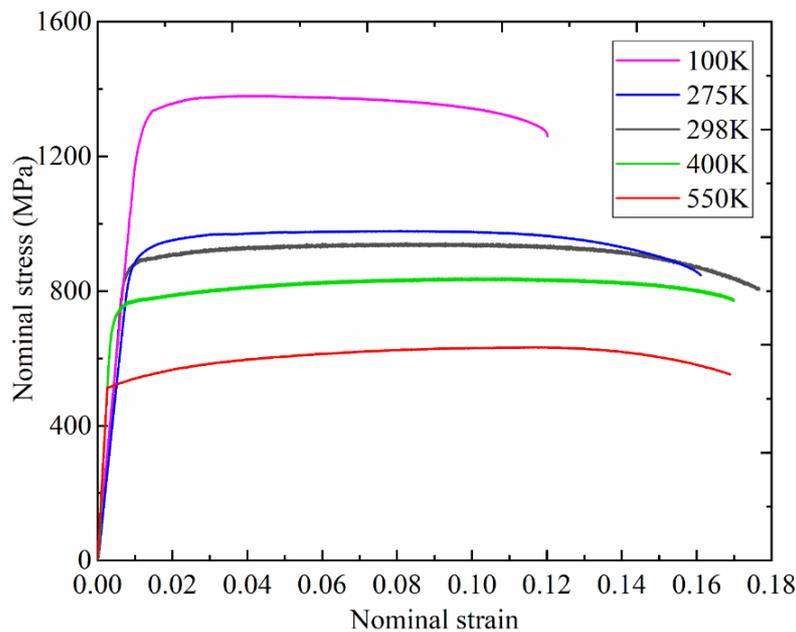
Figure 2.5 Nominal stress-strain curves at different temperatures.
