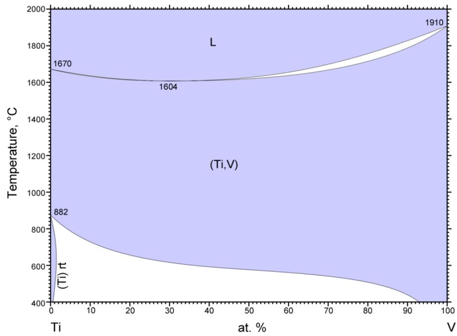
Figure. 1.13. Phase diagram of Ti-V [76].
