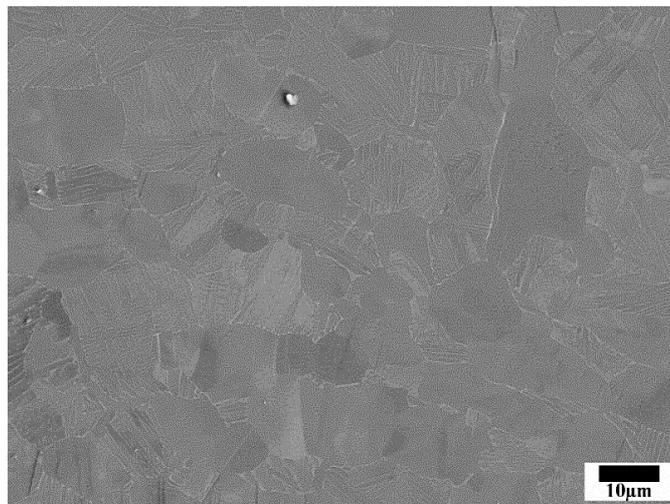
Figure 3.1. Microstructure showing slip traces at 0.5% strain.
