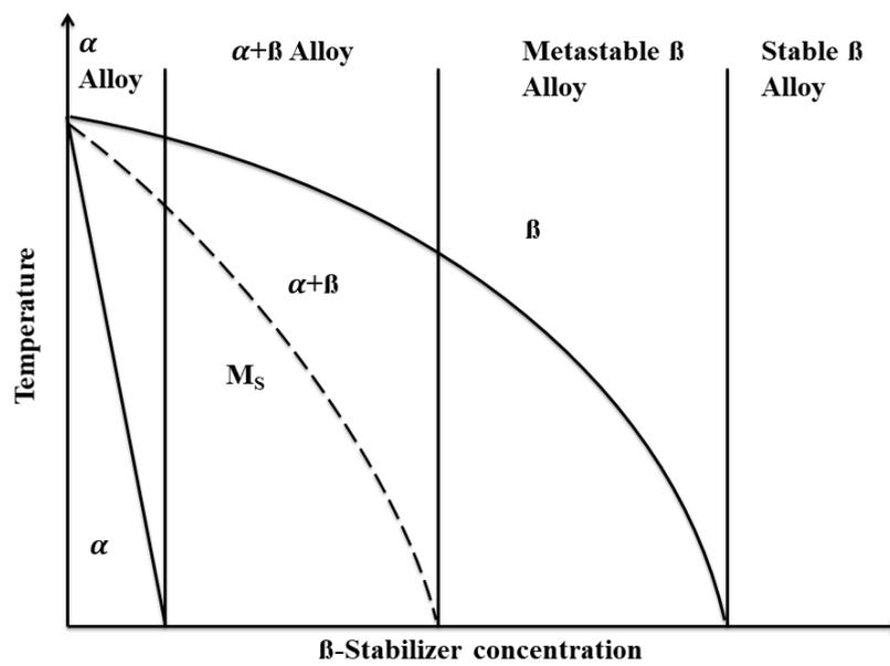
Figure. 1.12. Pseudo-binary section of  $\beta$  isomorphous phase diagram.
