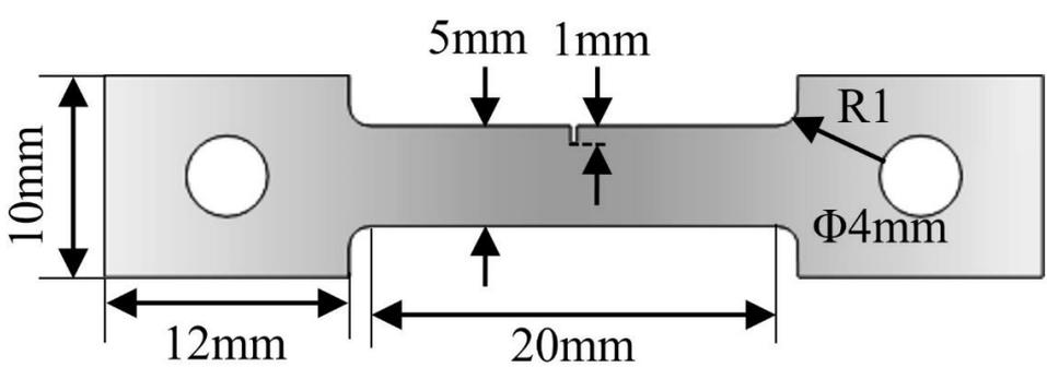
Figure 4.3 Schematic of a specimen for fatigue tests.
