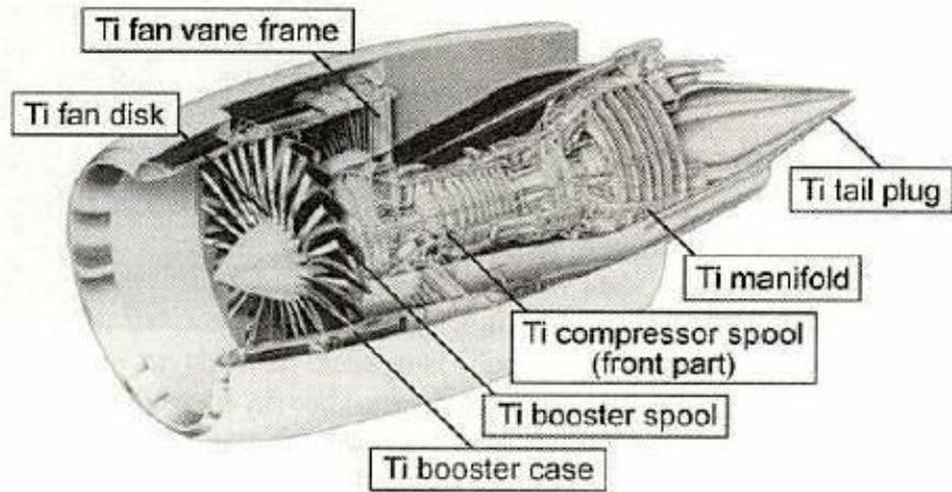
Figure 1.1. Titanium usage in GE-90 aero-engine [5].
