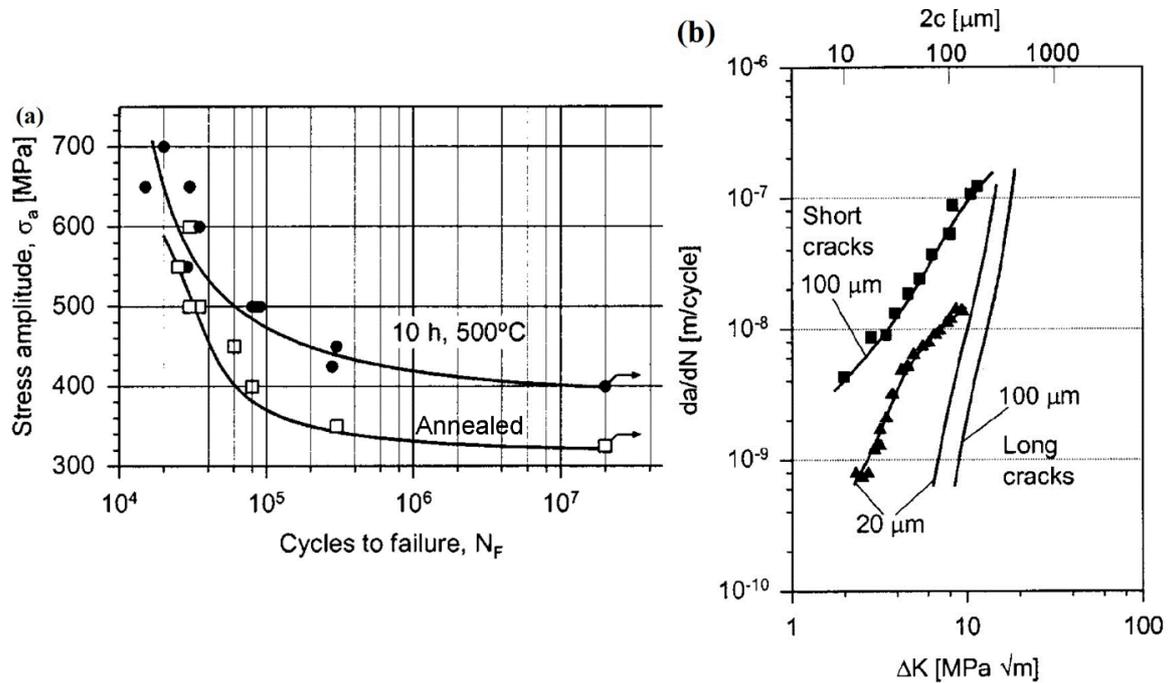
Figure. 1.22. Fatigue behavior of Ti-8.6Al. (a) Stress – Number of cycles to failure (S-N) curves from Ti-8.6Al, where one specimen was aged at 500 °C for 10 hours. The test was performed with  $R = -1$  [122], (b) Crack growth rates of micro (short) and macro (long) cracks [127].
