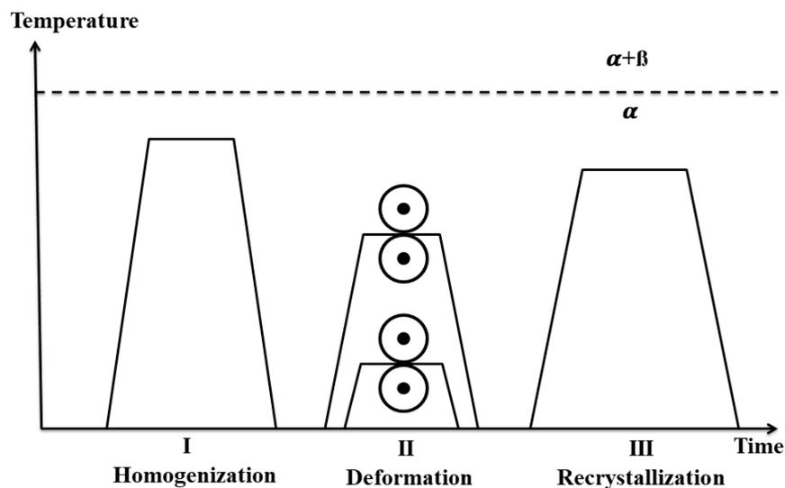
Figure. 1.7. Processing steps in the production of CP-Ti and  $\alpha$  Ti alloys.
