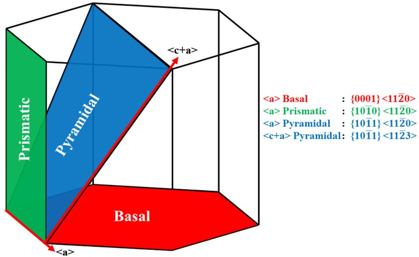
Figure. 1.8. Possible slip systems in alpha phase
