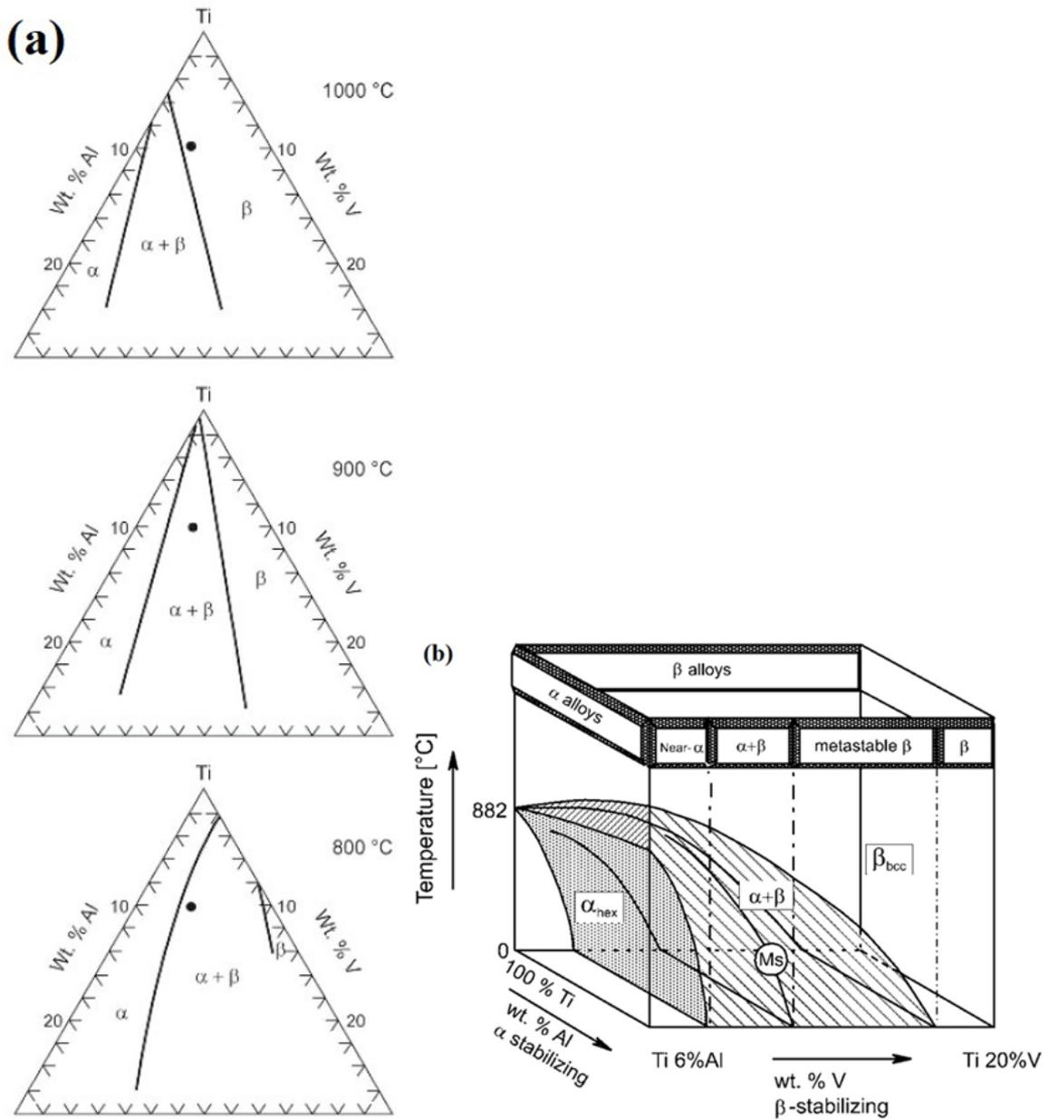
Figure 1.15. Ternary phase diagrams of Ti-Al-V. (a) Isothermal sections at 1000°C, 900°C, and 800°C through the Ti-rich corner of the ternary where Ti-6Al-4V composition with solid points are indicated [97], (b) 3D phase diagram to classify Ti alloys pertaining to Ti-6Al-V [53]
