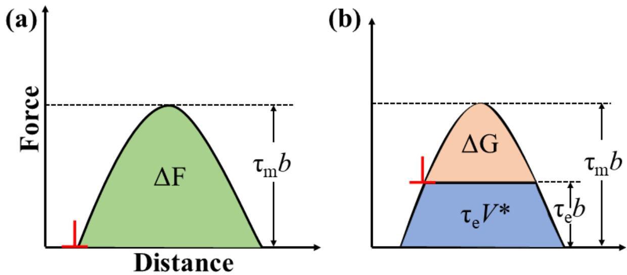
Figure 2.8. Schematic drawings of force on a dislocation when the dislocation overcome a short-range obstacle as a thermally activated process; A dislocation is represented as  $\perp$ . (a) Without applied stress, (b) with applied stress.
