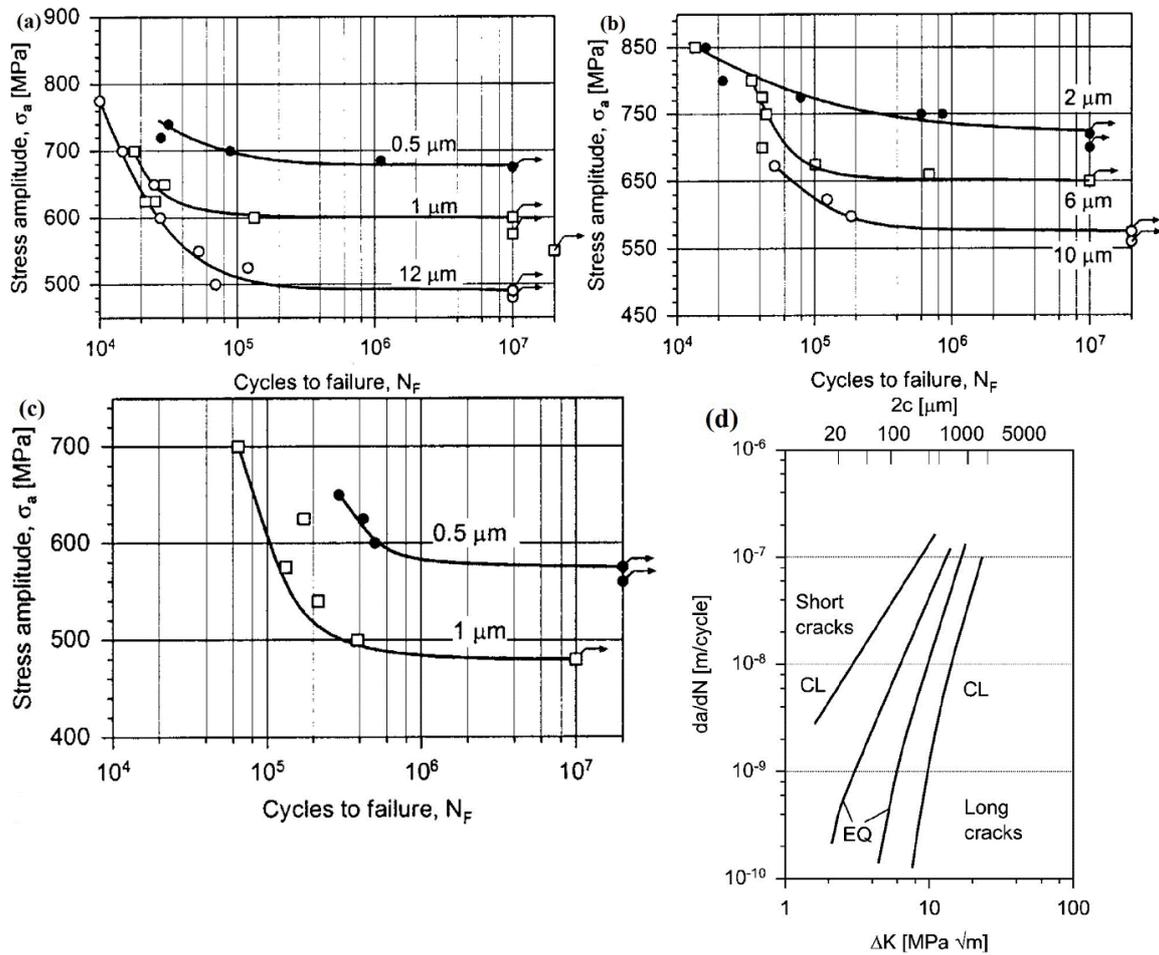
Figure 1.23. Fatigue behavior of Ti-6Al-4V containing different microstructural effects under HCF ( $R = -1$ ). (a) Effect of lamellae width in lamellar microstructure [130], (b) effect of  $\alpha$  grain size in equiaxed microstructure [130], (c) effect of lamellae width in duplex microstructure [131], (d) influence of micro and macro cracks on fatigue crack growth in Ti-6Al-4V with coarse lamellar (CL) microstructure and equiaxed (EQ) microstructure [132].
