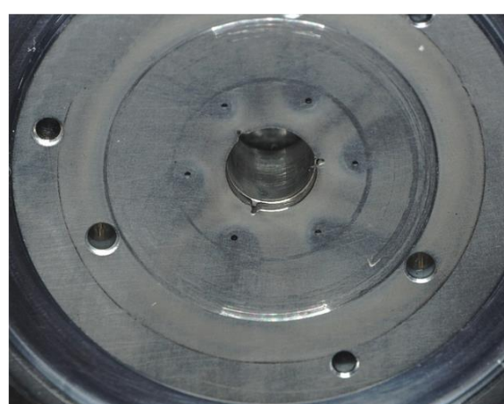
Radial Bearing [Turbine side]
