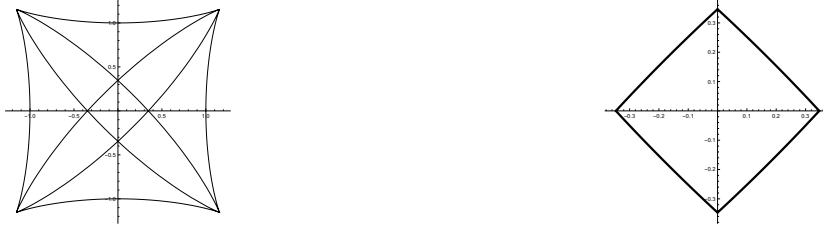
Figure 1.3: The image \xi_\gamma(S^1) of the Cahn-Hoffman map (left) and the Wulff shape W_\gamma (right) for \gamma defined by (4.1). W_\gamma is a subset of \xi_\gamma(S^1) .
