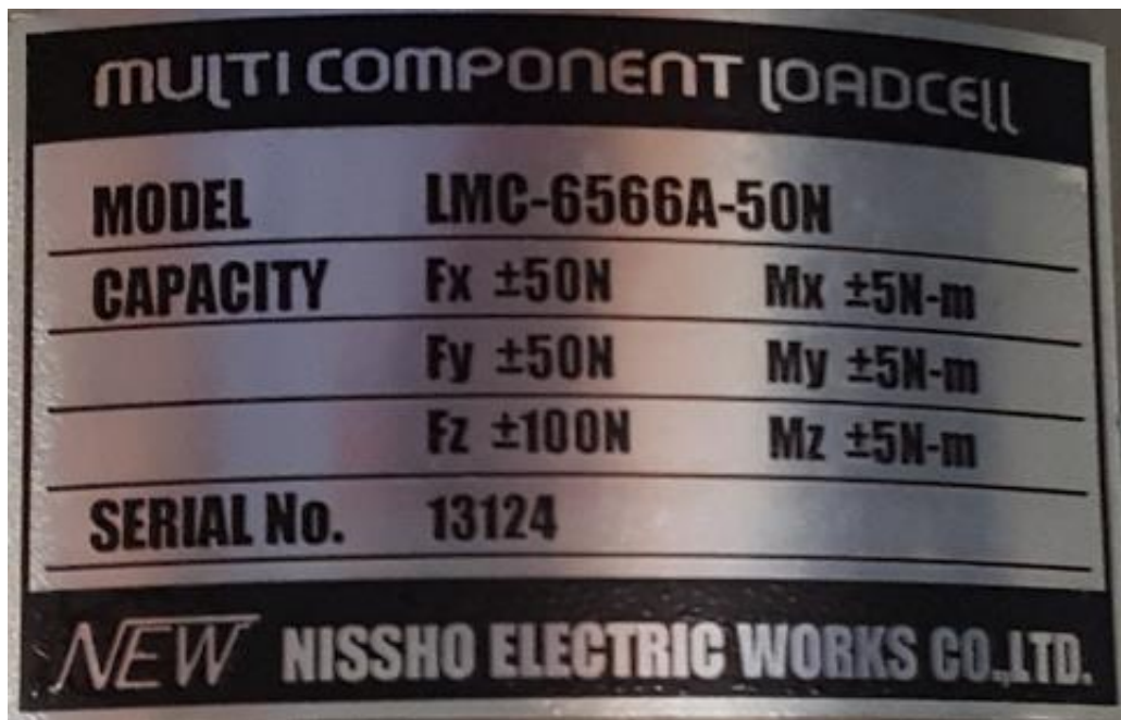
Figure 3.6 Model number and capacity of the load cell [60].
