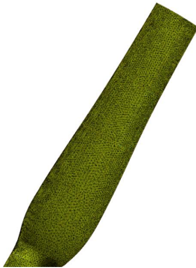
Figure 4.5 Surface mesh of the fully resolved wind turbine rotor.
