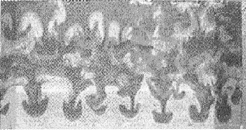
Fig. 3 Experiment of RTI with the Vessel of 0.4 \times 0.2 \times 0.02 m in Size.
