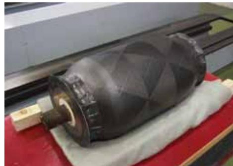
**Fig. 19** The third FW tank after Cure.
