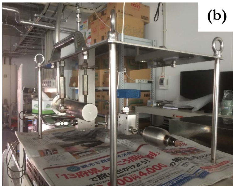
Figure 3.2-2 Photographs of the experimental setup; (a) The thermal bath; (b) the isochoric cell
