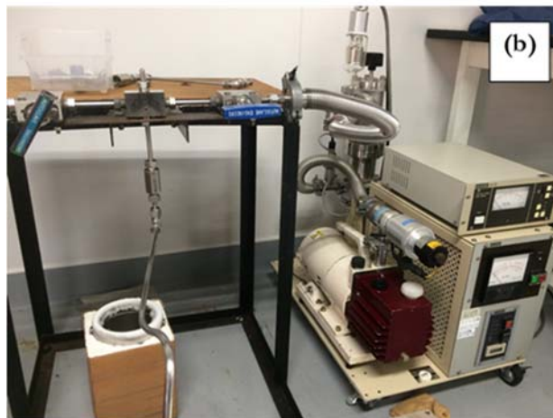
Figure 3.2-6 Figure of the vacuuming process in which; (a) the isochoric cell is connected to the tubing port; (b) vacuum is connected to the port as well and started
