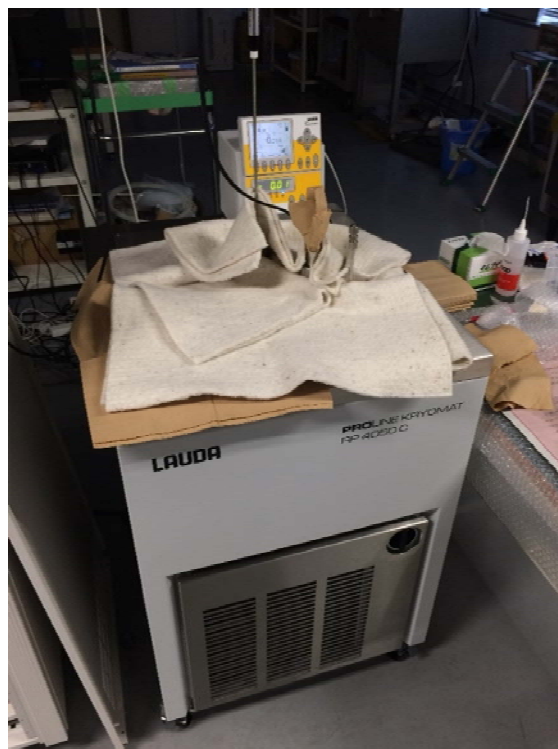
Figure 3.2-9 Current insulation method for the heat leaks through the top panel use insulative cloth in addition to the layer on insulative material present
