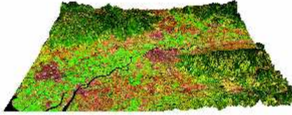
Figure 3: Landsat 5 TM false color composite image in Chikushi plain, Japan, acquired on April 24, 1997. The image displays band 5 as red, band 4 as green and band 3 as blue. Bird's eye view.
