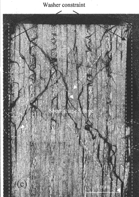
Figure 11 Microphotographs of the bearing failure of a mechanical joint at -100^\circ\text{C} (a) Pinned joint, at 40N-drop point [11] , (b) Bolted joint, at the knee point (21.91 kN) and (c) Bolted joint, at the first maximum point
