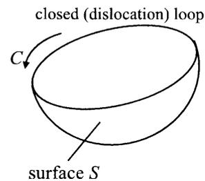
Fig. 2 Closed (dislocation) loop  $C$  bounding a surface  $S$ .
