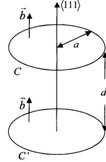
Fig. 3 Two coaxial circular dislocation loops,  $C$  and  $C'$ , located on  $\{111\}$  plane. Burgers vectors of the two dislocation loops  $\vec{b}$  are assumed to be parallel to the  $\langle 111 \rangle$  direction.
