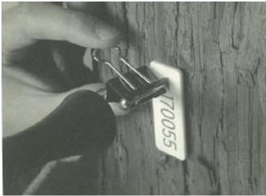
Fig. 4-1 Driving a nail in to the stem (Yoshida, 2007).
