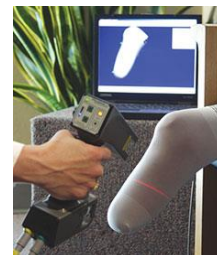
Fig. 2.1 Example of 3D scanning process for the stump [4]
