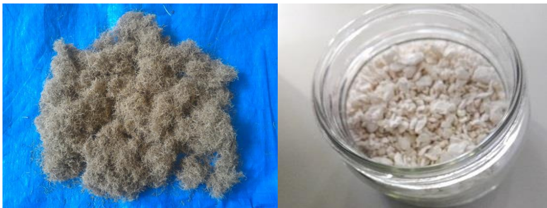
Figure 2.1. Optical image of empty fruit bunches fibers (left) and its bleached pulp (right)
