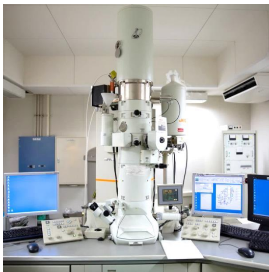
Fig. 2.4. Transmission Electron Microscope (TEM, JEM-ARM 200F, JEOL Co., Japan).
