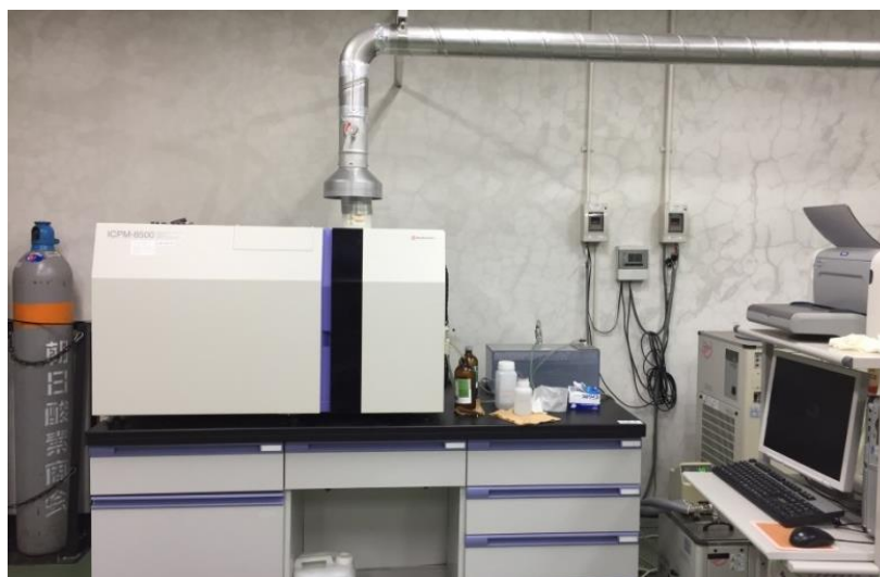
Fig. 2.8. Inductively Coupled Plasma Mass Spectrometry (ICP-MS, model: ICPM-8500, Shimadzu Co.).
