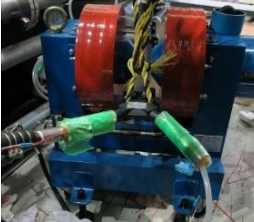
Fig. 92 The final design of the water load, waveguide and the electromagnet
