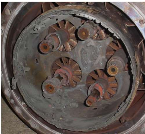
Figure I-5 burner assembly damaged by combustion instability [6]
