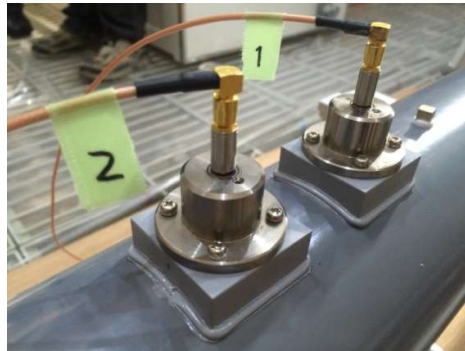
Figure IV-5 Installation of microphones
