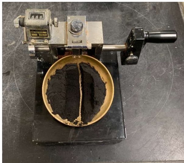
(a) Sample's preparation for Liquid Limit test
