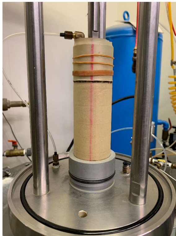
Photo 6.1 Bender elements were set up in the identical direction by datum line marked in rubber membrane.
