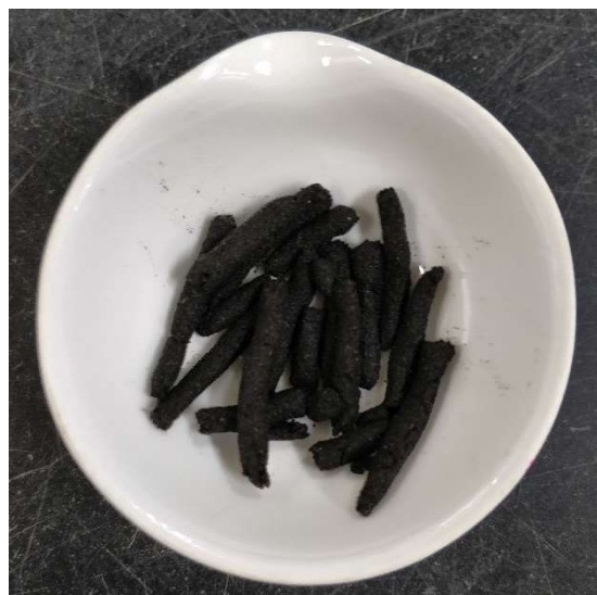
(b) Sample's preparation for Plastic Limit test
