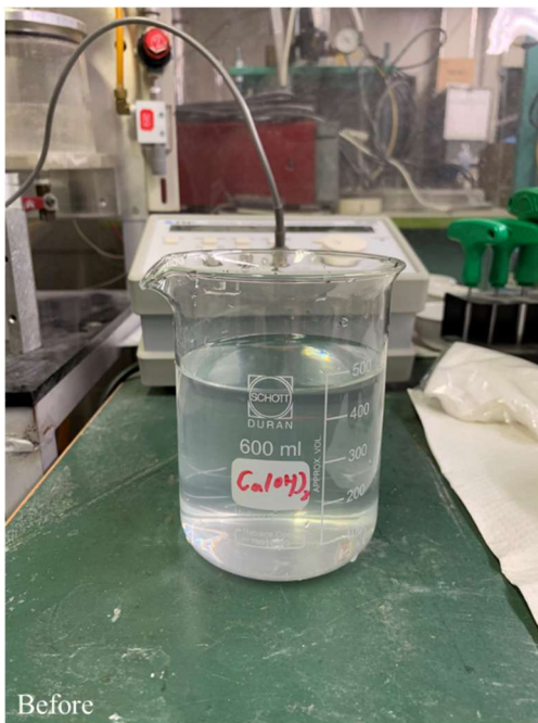
Photo 3.3 Solution of \text{Ca}(\text{OH})_2 before and after filling with \text{CO}_2 in specimen
