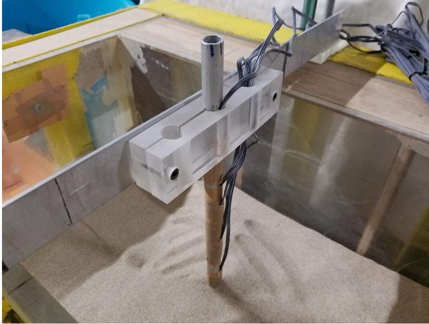
Figure 3-13 Pile model clamping on a guide bar during soil setup
