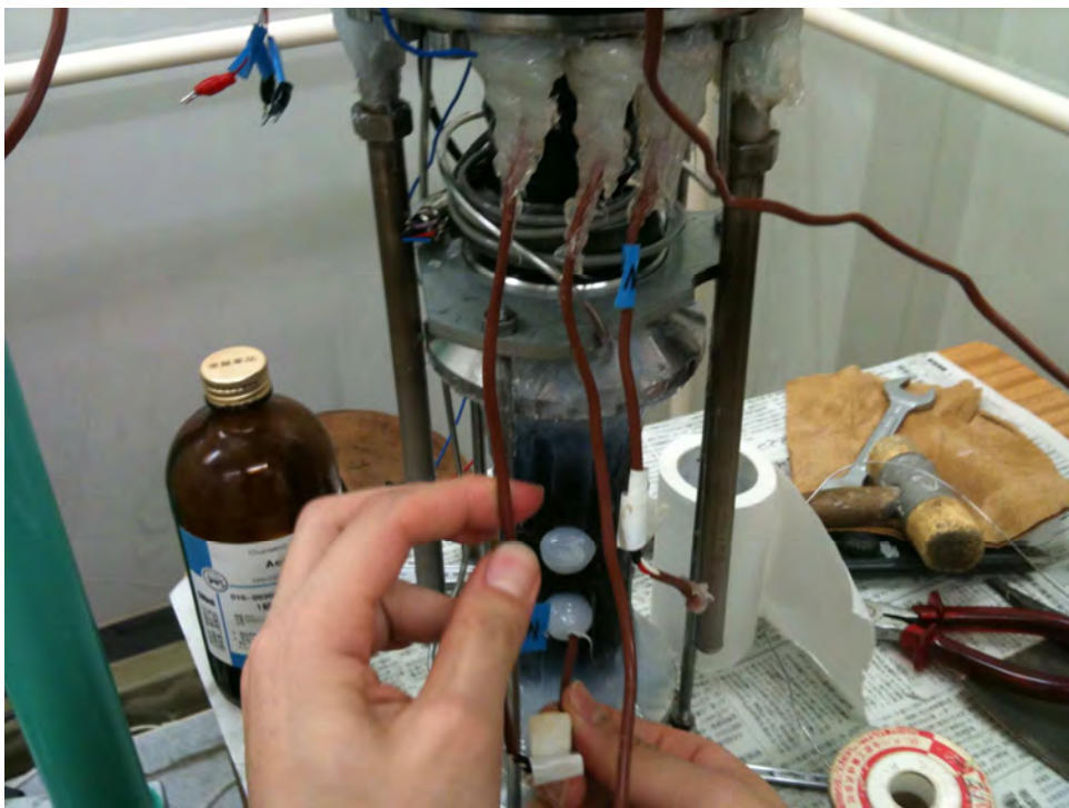
Figure 3-19. Installing of strain gauges and silicon coating.
