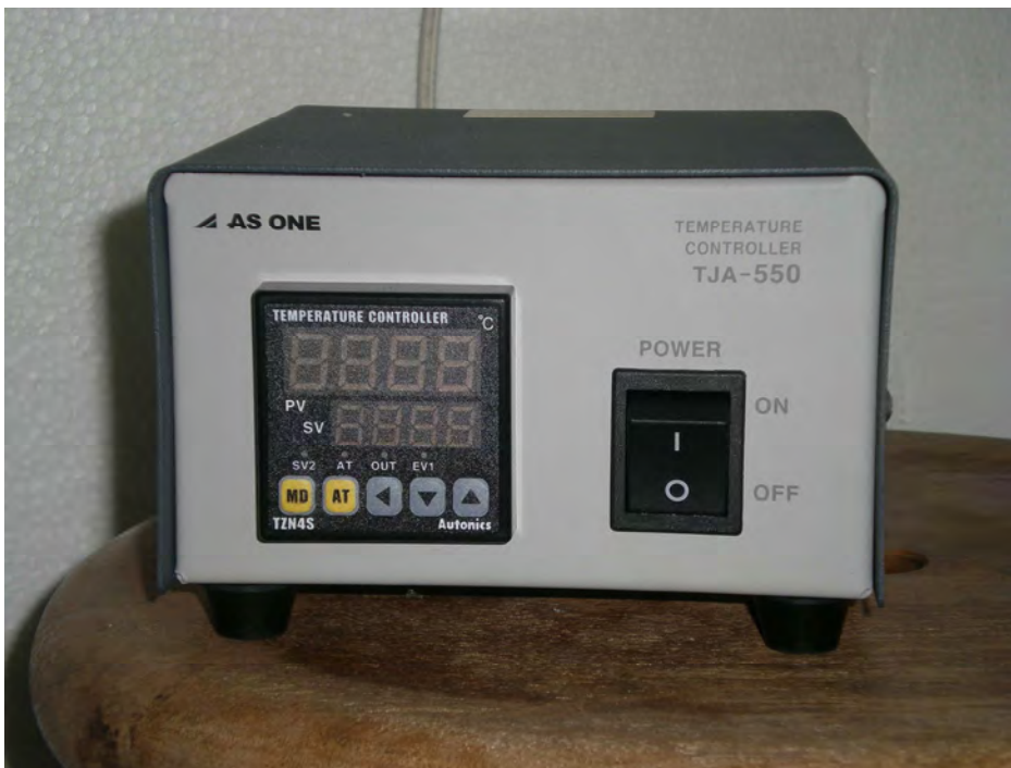
Figure 3-12. Temperature controller for pressure vessel.
