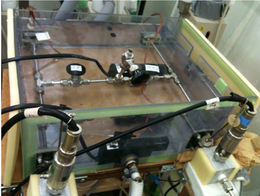
Figure 3-9. Water bath for controlling temperature of syringe pipes.
