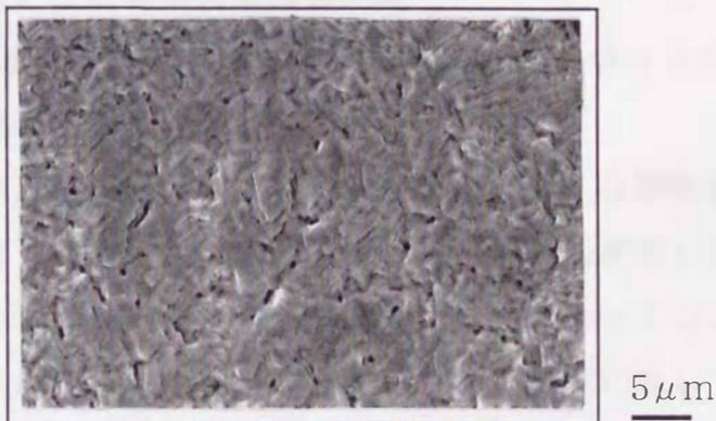
Fig.4-9 Effect of current density at initial stage on morphology of electrodeposited Zn.
