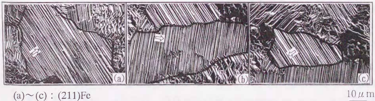
(a)~(c) : (211)Fe 10\mu\text{m} Fig.2-4 Surface morphology of Zn electrodeposited on (211)Fe plane. ( 50\text{A/dm}^2 , 20\text{g/m}^2 )
