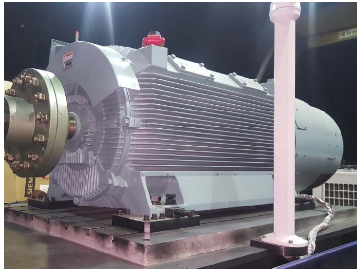
Fig. 4.10 The induction motor for rotating the metal billet using spindle unit
