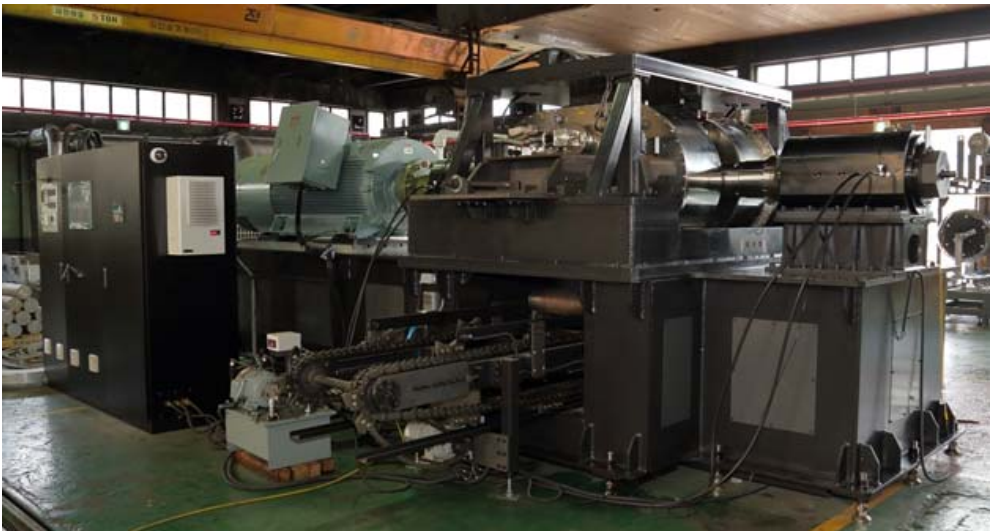
Fig. 5.18 The SIH for test of the performance analysis of various metal billets
