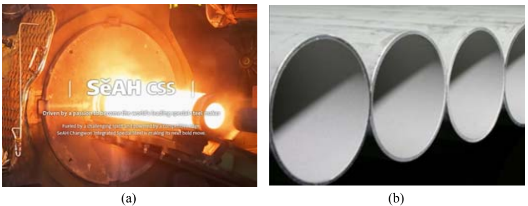
Fig. 1.2 (a) Extrusion process for stainless steel pipes and tubes; (b) An example of extrusion parts, pipes and tubes for plants (photos from SeAH CSS homepage;www.seahss.co.kr)
