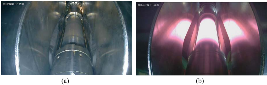
Fig. 5.23. (a) A picture of the STS billet on the specific position to be heated; (b) after finishing the heating process of the STS billet
