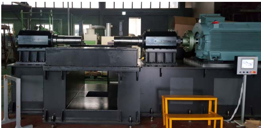
Fig. 4.2 The installation of the rotational motor and the spindle unit with hydraulic system of a SIH
