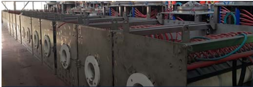
Fig. 1.17 Conventional induction heater has each coil against a diameter of the metal billet and needs a big space for storage of various copper coils
