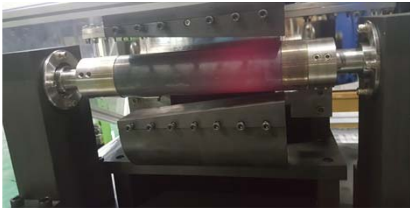
Fig. 1.15 10 kW SIH heating results for the magnetic control along the longitudinal direction.
