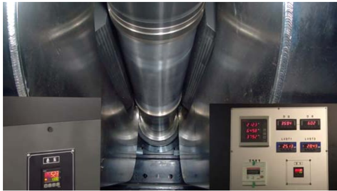
Fig. 5.19 A picture of an heated aluminum billet of a SIH operation at specific time
