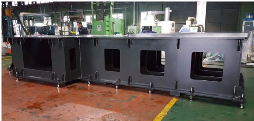
Fig. 4.1 The supporting base installation of a SIH
