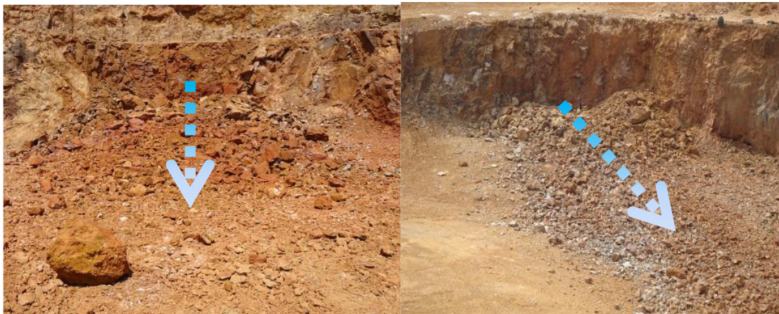
Fig. 4.13 The difference of flight distance of blast-induced fragmented rocks
