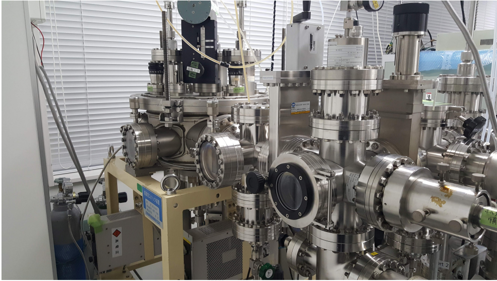
Figure 3.2: DC/RF Sputter machine with several sources out of which we used Pt and W for the following experiments
