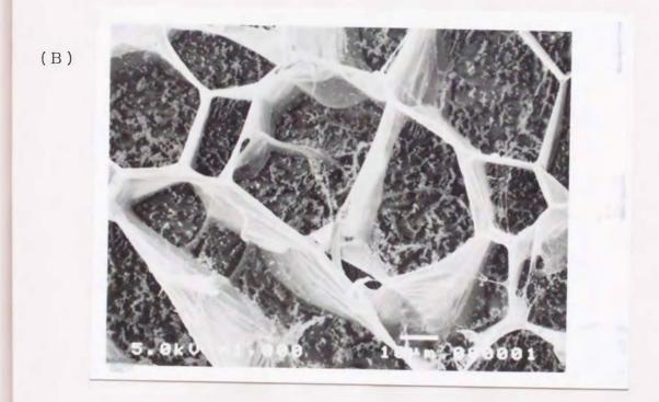
Fig. 6.2 CRYO-SEM photographs of hydrogel of P/PULP-AM-Hyd(Sample B). Scale bars represent 100  $\mu m$  in (A) and 10  $\mu m$  in (B).
