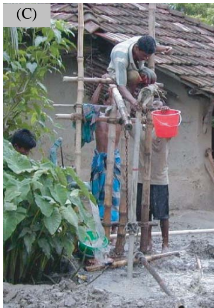
Figure 2.2 Photograph of the sampling: (A) Sediment collection using pressure boring, (B) Sediments in a collection tube, (C) Sediment collection using local boring method, (D) Collected sediments in a rack, and (E) Groundwater sampling from wells
