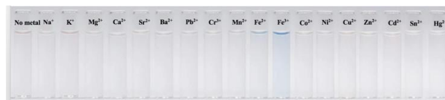
Fig. 1. Color change on the presence of one equivalent of metal ions in spirooxazine solution in 1,4-dioxane.
