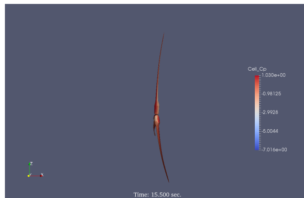
Figure 3-8: Out-of-plane aeroelastic bending effect on the NREL 5MW HAWT using MIRAS-FLEX.
