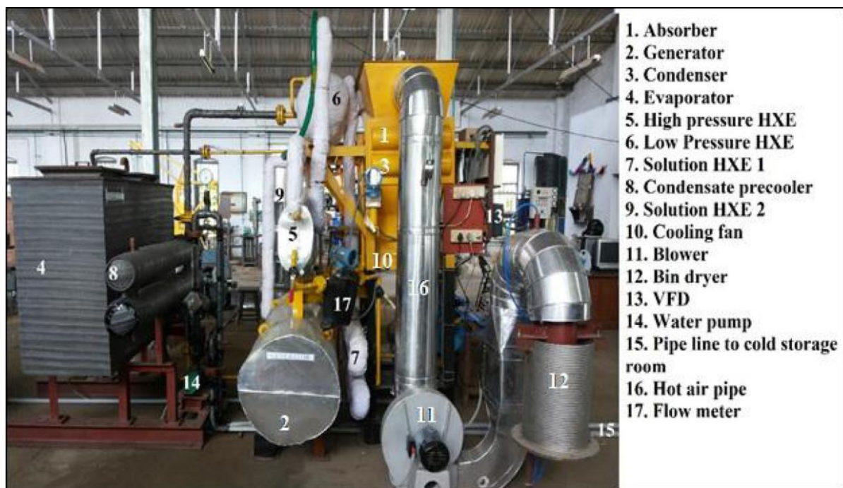
Figure 2.10 Air cooled vapour absorption system with attached bin dryer (Sivakumar et al. 2016).
