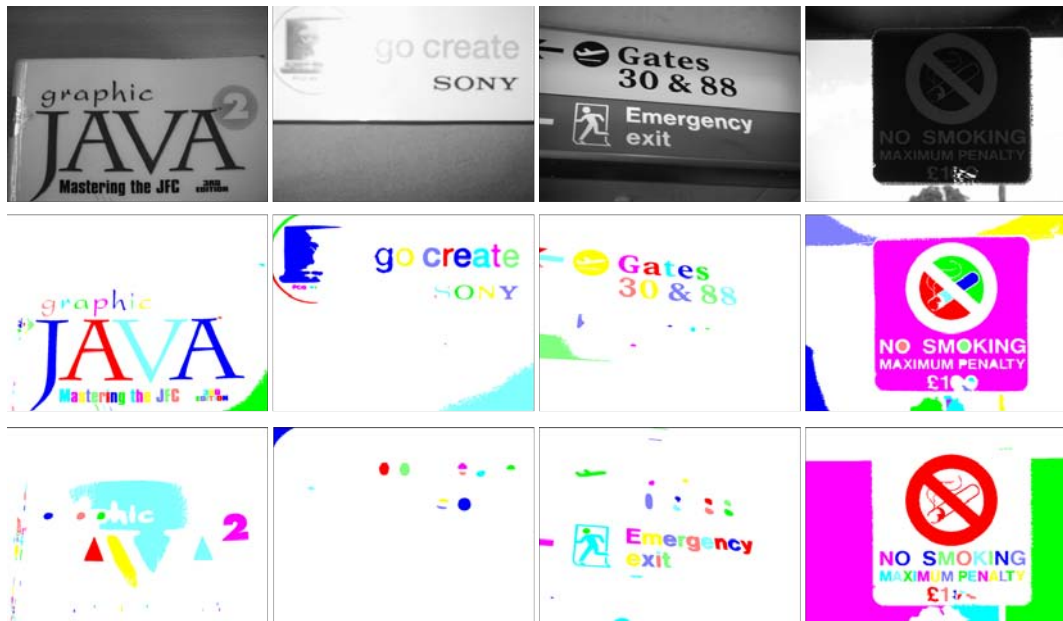
FIGURE 3.11: The results of extracting text characters from different images by using the MSER method. The images on the first, second, and third rows are the gray image, the extracted black text characters, and the extracted white text characters, respectively.
