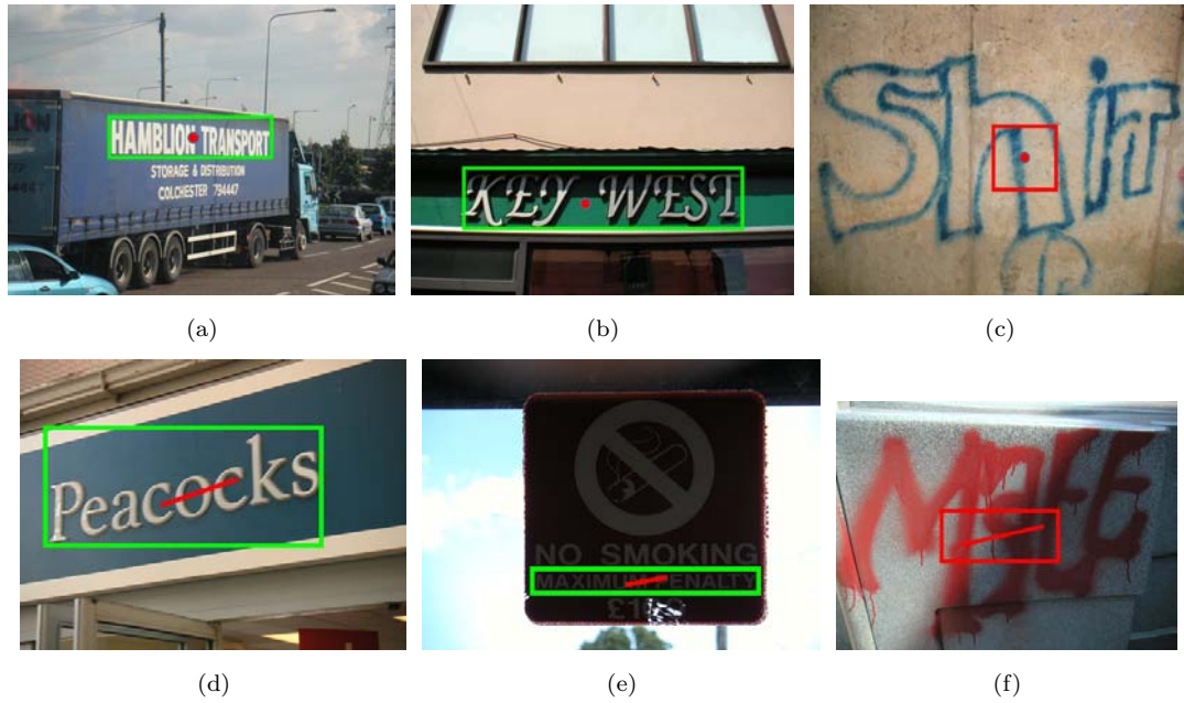
FIGURE 2.6: Successful and failure examples of text line extraction with user-intention on the ICDAR2003 competition database.
