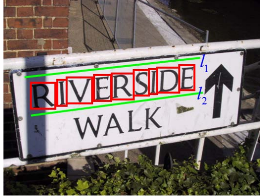
FIGURE 2.5: Global constraint for user-intention text line between two green parallel lines l_1 and l_2 .
