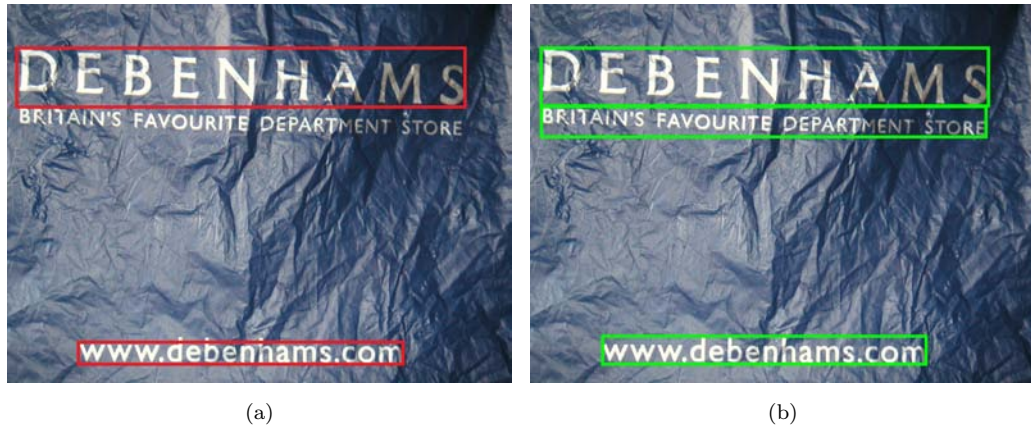
FIGURE 5.5: Text line extraction results of (a) gray channel k-shortest paths optimization and (b) multi-channel k-shortest paths optimization method.
