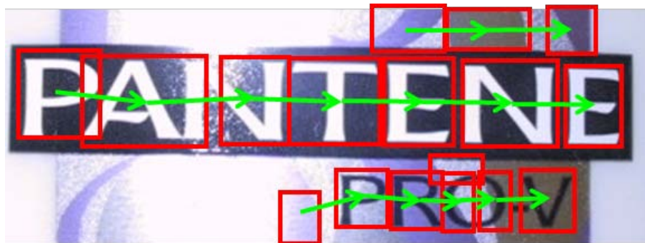
FIGURE 3.1: Construction of the directed graph based on the spatial arrangement of connected components.
