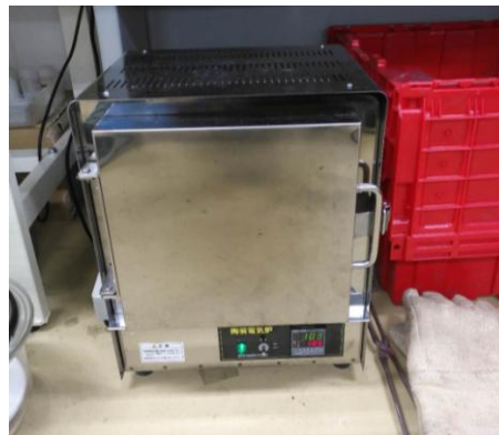
Figure 2-5. Electric high-temperature furnace for coal composition measurement.
