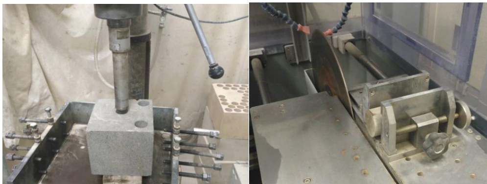
Figure 2-2. Coring bit (Left) and surface grinder (Right).
