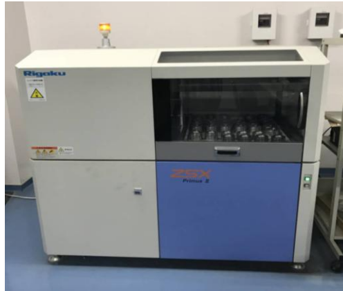
Figure 2-4. X-ray fluorescence equipment for rock composition measurement.
