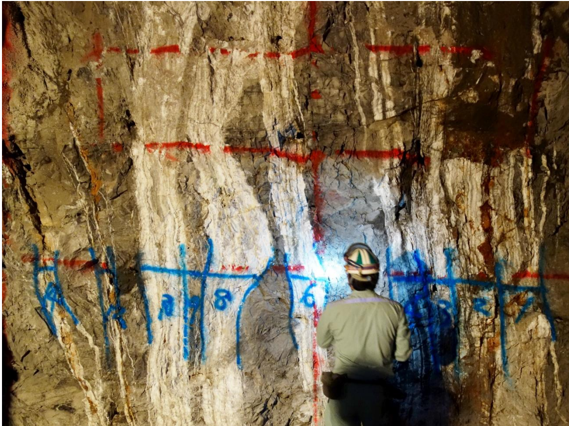
Fig. 2-2 Illustration of a mining face in the Hishikari mine (within the Yamada sub-deposit). The scale is provided by the person standing.
