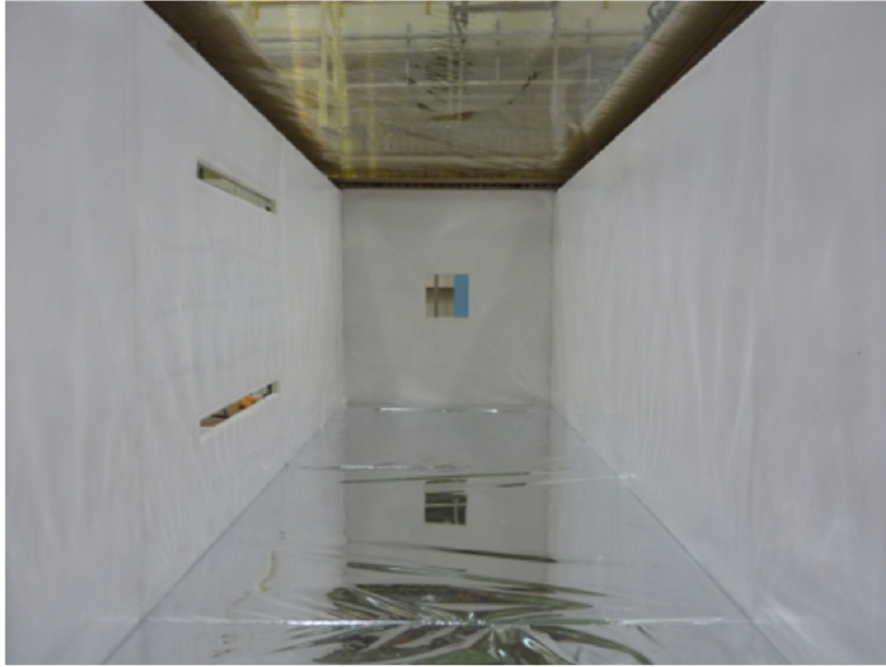
Figure 2.12: Inside photograph of the TPC. There are two slits on one side of the TPC for calibration.
