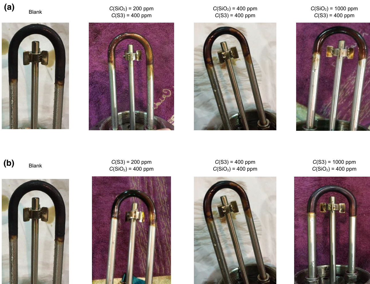
Fig. 6 Physical appearance of the deposited wax from treated crude oil at various concentrations. a Cold finger U-tube treated by SN3 with different concentrations of SiO 2 nanoparticles, b Cold finger U-tube treated by SN3 with different S3 concentrations
