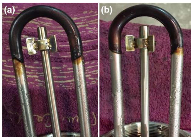
Fig. 10 Photographs of wax deposition on the cold finger after 15 h of treatment on both blank and SN3-treated samples. a Blank sample after 15 h, b SN3-treated sample after 15 h
