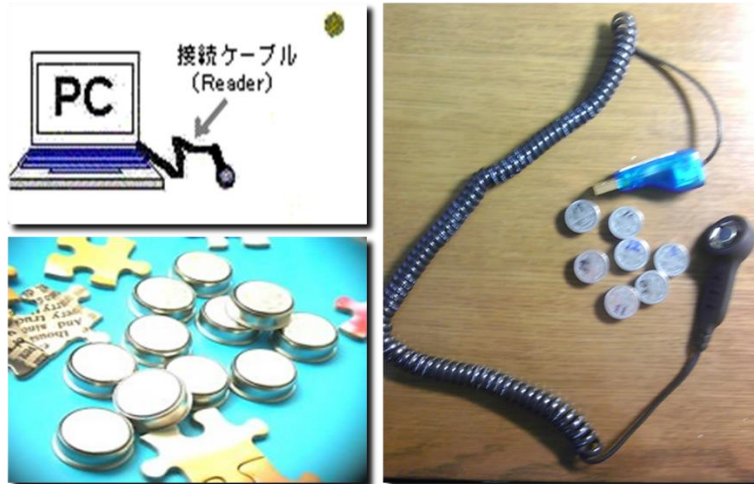
Fig. 4.5. The Hygrometer sensor for the measurement of dry bulb temp. and RH%. Source: (KN. Labs 2010)
